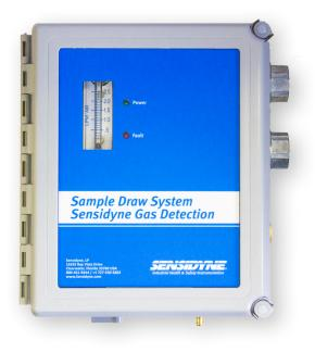
The Sensidyne Sample Draw System samples air from remote locations pulling a sample to gas detection transmitter(s) and is offered as a diaphragm pumped or an air operated aspirator unit. It is designed for placement in a Class I, Division 2 Hazardous (Classified) area to sample from a Class I, Division 1 Hazardous (Classified) area, Groups C and D. A Division 2 approval eliminates the need for flame arrestors and reduces related maintenance caused by dirt and moisture.
